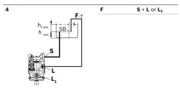
For NG45 and NG63 series 52, L<sub>1</sub> is opposite, L must then be connected if necessary.
