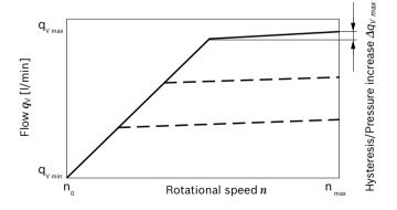
Characteristic curve valid at  $n_1$  = 1500 rpm and  $\theta_{fluid}$  = 50 °C.
