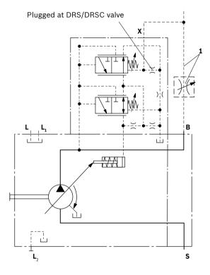
**1** The sensing orifice (control block) and the line is not included in the delivery contents.
