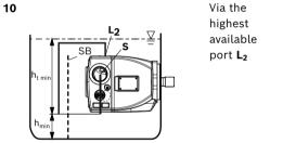
Automatically via the open port L2 due to the position under the hydraulic fluid level
