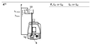
Because complete air bleeding and filling are not possible in this position, the pump should be air bled and filled in a horizontal position before installation.
