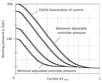
Characteristic curve measured with pump in zero stroke Further information on request.
