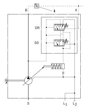
1 The metering orifice (control block) is not included in the scope of delivery.
